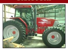
McCormick MTX135 FWA Tractor w/Triple Hydraulics, 18.4X42 & 14.9X30 Tires, 90% Rubber, 1,380 Hrs. Nice
